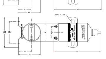
790104-1...... 4+1 magnets, 7.45" diameter 790114-1...... 4+1 magnets, 5.00" diameter .480 (12.19) DIA .475 (12.06) MAGNETS ARE INSTALLED NORTH POLE FACING DUT. 5.005/5.000 DI (127.1/127.0) .375 (9.5) 790105-1..... 5+1 magnets, 7.45" diameter MAGNETS ARE INSTALLED WIT NORTH POLE FACING OUT. 790115-1..... 5+1 magnets, 5.00" diameter 790106-1...... 6+1 magnets, 7.45" diameter
